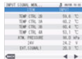
Indication of Internal Signals
