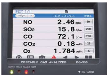
Front panel LED's clearly display unit status/recording data
